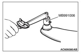
Move the lower arm ball joint stud back and forth for several times, and measure the lower arm ball joint rotation starting torque using special tool MB991006.
