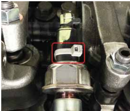
Cable tie location
