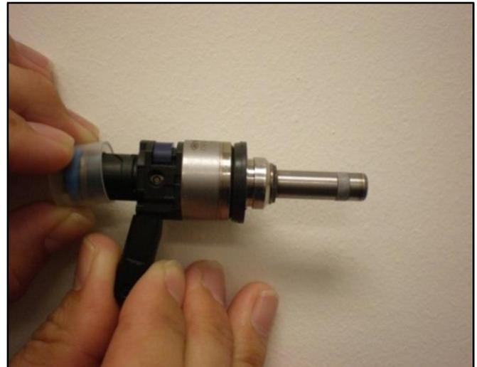
10. The stepped rubber side of the seal goes towards the injector.
