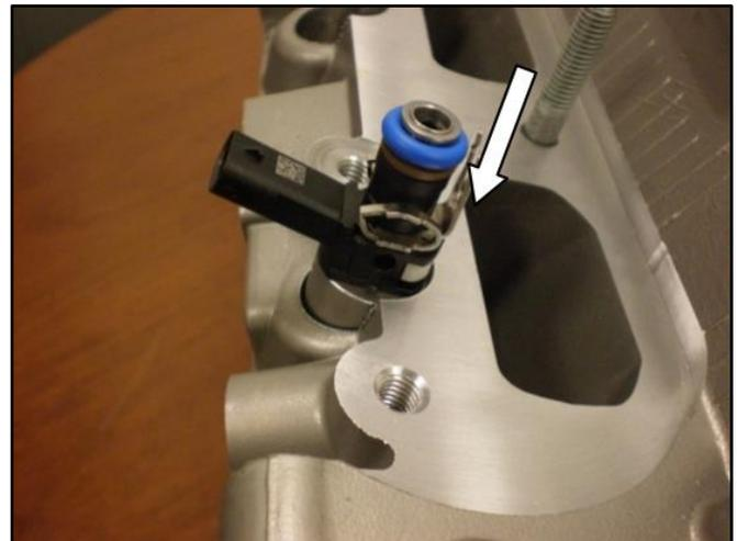
7. Twist slightly while pressing the injector into position in the head.
