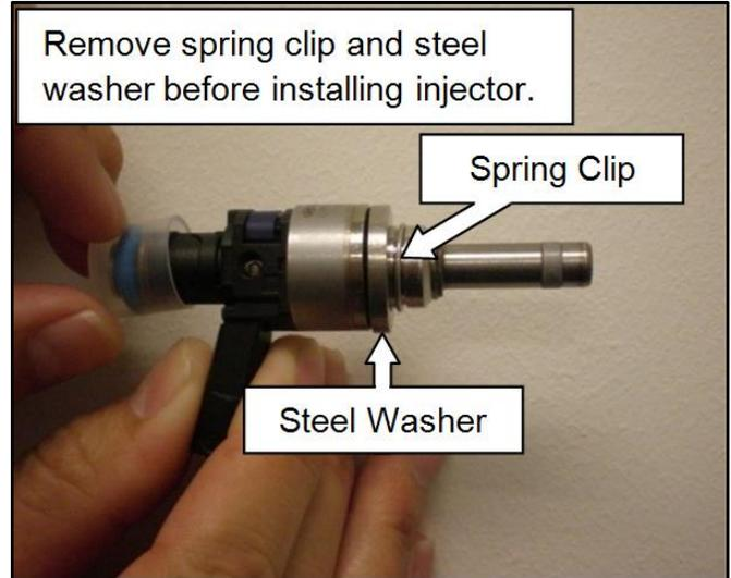
9. Install the washer seal onto the injector with the rubber side (stepped) toward the injector.
