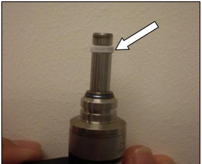
5. Place the resizing tool (flange up) over the seal. Twist the tool slightly while pushing down over the seal. This should reduce the size of the seal.
