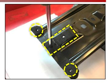
5. Apply felt tape at the four (4) crossmember mount locations and carefully poke a small opening through the felt tapes, as shown (C) for ease of retaining bolts installation.
