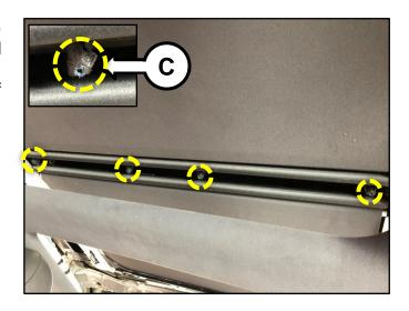
Apply LOCTITE® 242 or equivalent medium strength threadlocker to the crossmember retaining bolts and immediately reinstall the felt-applied crossmember. Reinstall all removed components in the reverse order of removal.
