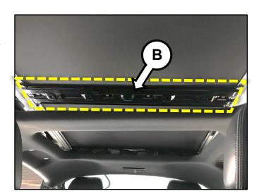
With the sunroof crossmember placed on a flat surface, facing down, apply felt tape to the highlighted areas.
