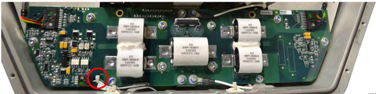
Figure 4. HVIL Circuit Card – Wire Tie Location
