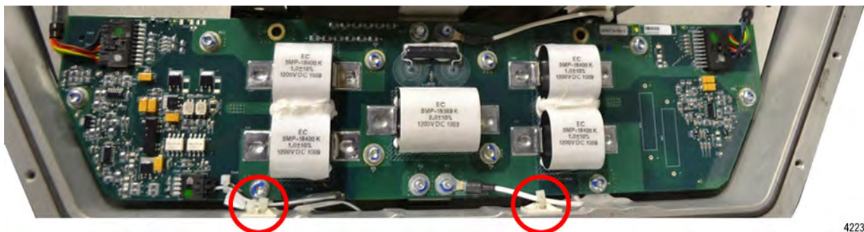
Figure 57. HVIL Circuit Card – Two (2) Wire Tie Locations
