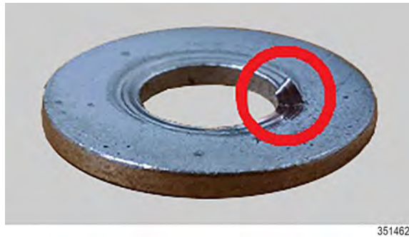
Figure 34. Burr on Flat Washer
