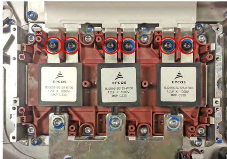
Figure 40. SKiM Module Fastener Locations
