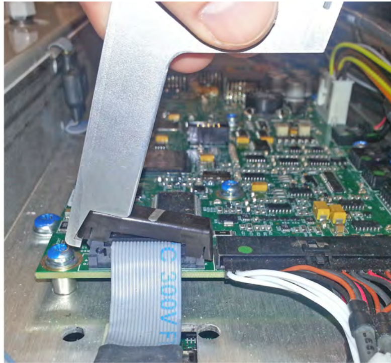
Figure 18. Cable Strain Relief Cap Removal (BCA Cable Card Connector Shown for Clarity)
