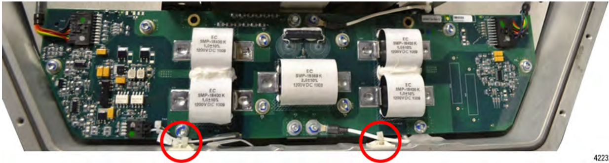
Figure 5. HVIL Circuit Card – Two (2) Wire Tie Locations
