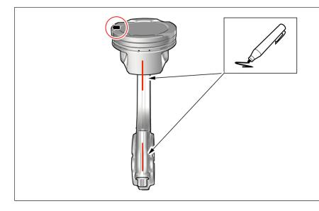
Caution! Note the position of the component before removal.
