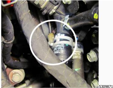
2. On Malibu (LFV engine) applications **only**, inspect the engine wire harness adjacent to the heater inlet hose for contact with the heater inlet hose clamp on the engine outlet portion of the hose as shown.
