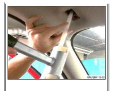
4. Using a suitable tool, such as a thick plastic wedge tool, reshape the sheet metal upwards using a mallet.
