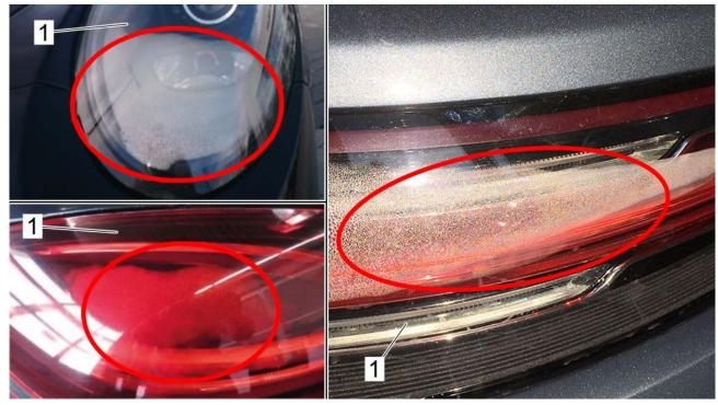
Level 3: Slight drops forming on lighting component
