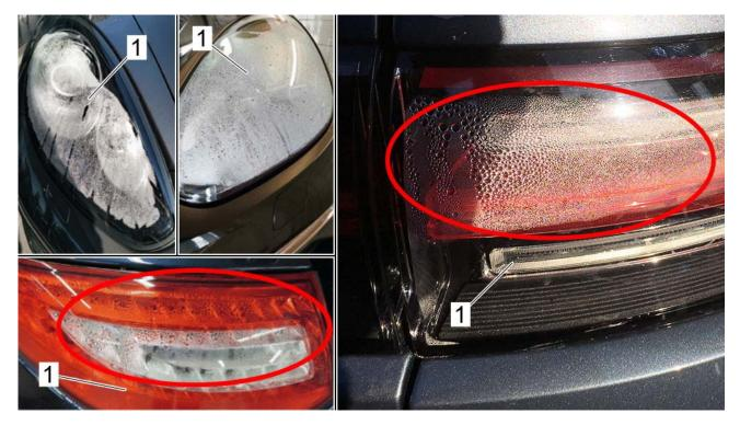
Level 4: Significant drops forming on lighting component
