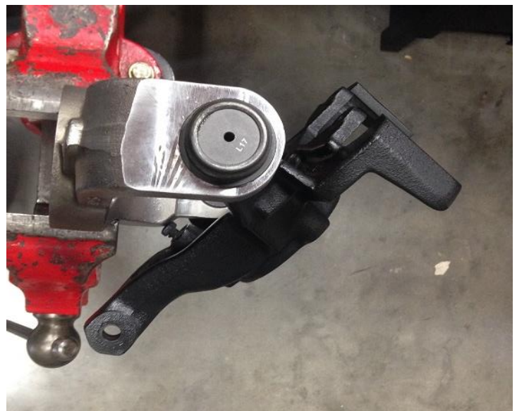
Image D - correct steering stop engagement.
