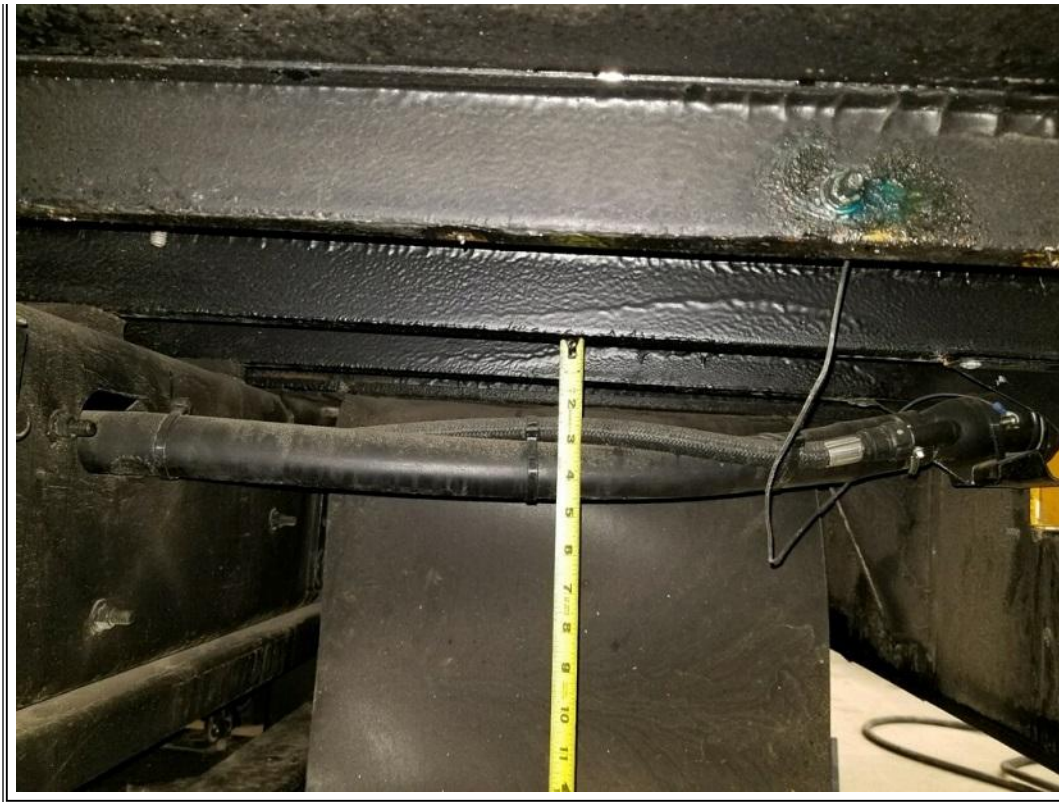
Figure 5 - Unacceptable Fuel Fill Hose Droop
