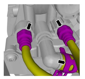
Undo the hoses from the connections.
