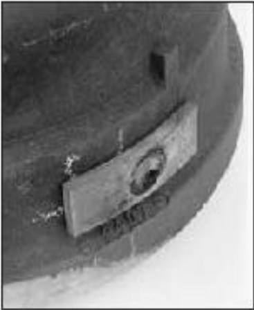
Welded balance weight
