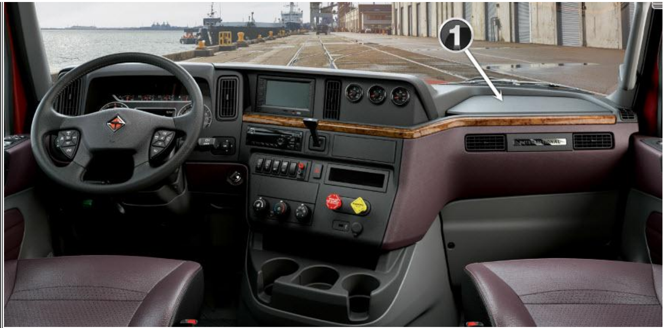
1. Fuse Panel Cover
