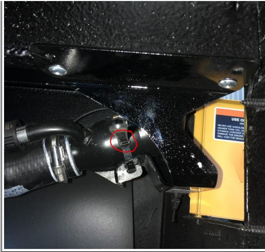
Figure 4 - Acceptable Fuel Fill Hose Droop
