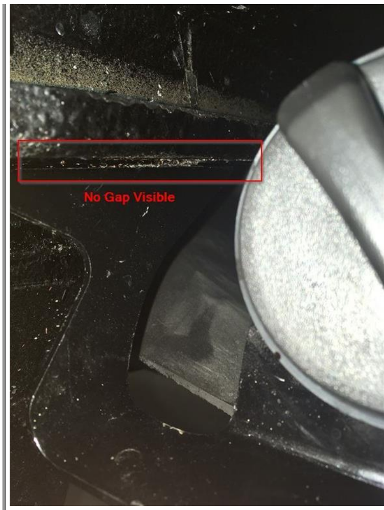
Figure 7 - Unacceptable Fill Receiver Bracket Gap
