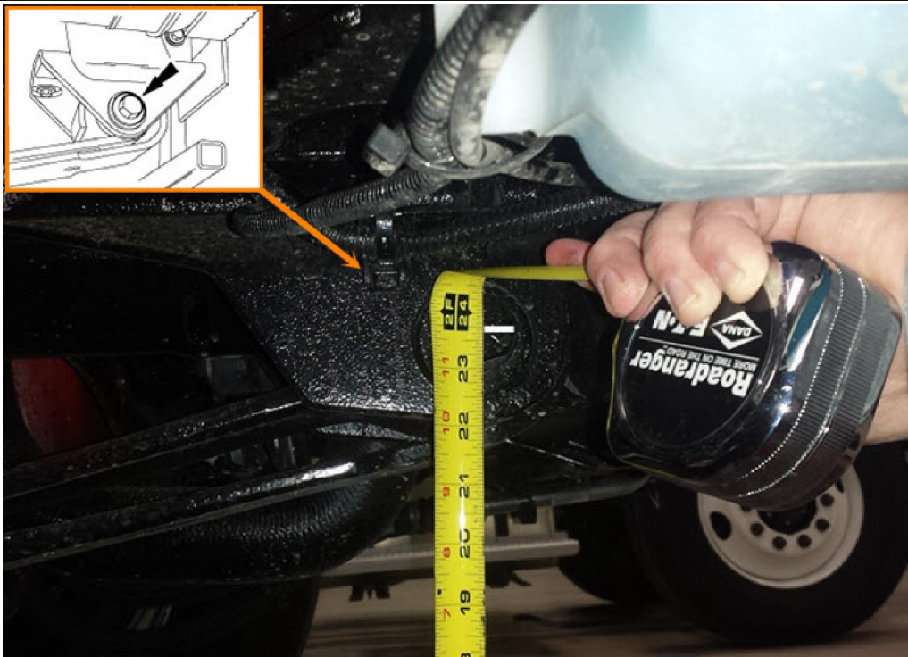
Figure 5 Left Front Spring Shackle Bolt
