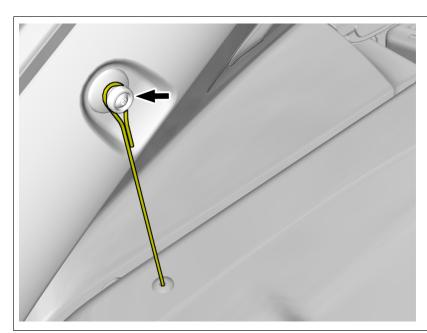
Loosen the marked detail. Repeat on the other side.
