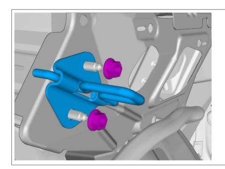
Install the marked component. Install the nuts
