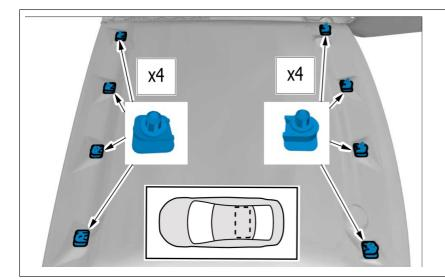
**Note!** Make sure that the mating faces are at a minimum temperature of 20°C.
