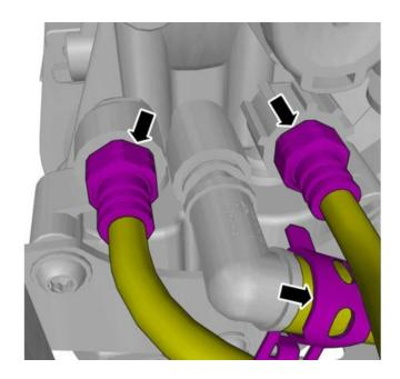
Undo the hoses from the connections.
