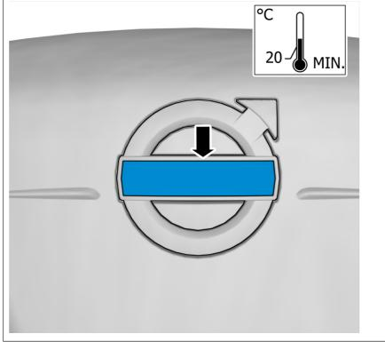
Caution! Make sure that equal pressure is applied to the full length of the component.
