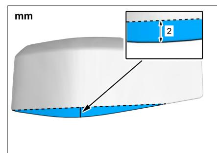
Measure and mark as illustrated. Remove the marked part. Even out the edge using a file.
