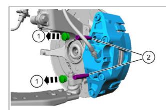
Warning! The brake caliper housing Torx bolts must not be removed.
