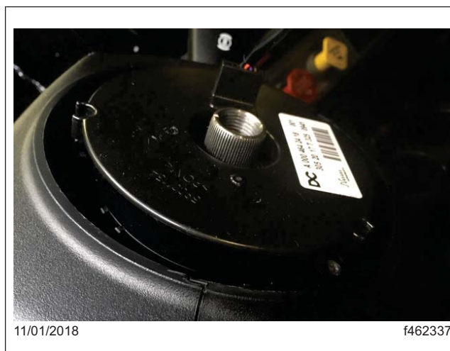
Fig. 5, Steering Column Splines with Undamaged Grooves
