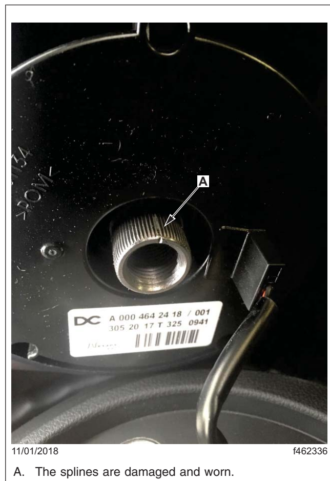
Fig. 4, Damaged Steering Column Splines
