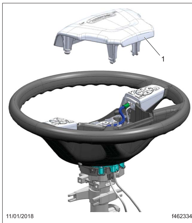
Fig. 3, Removing the Steering Wheel Cover
