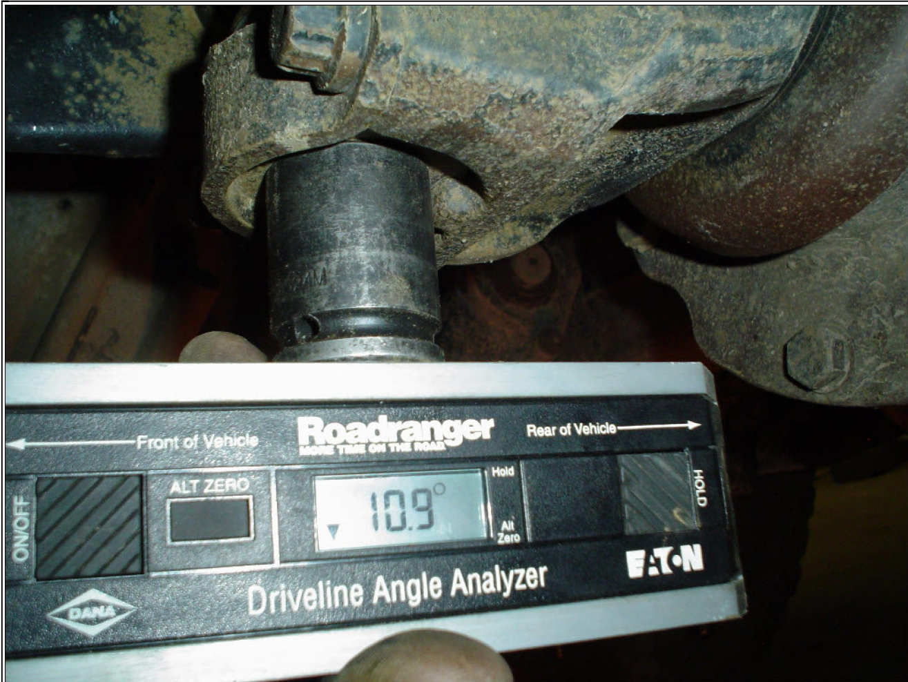
Figure 2 - Measuring Pinion Angle
