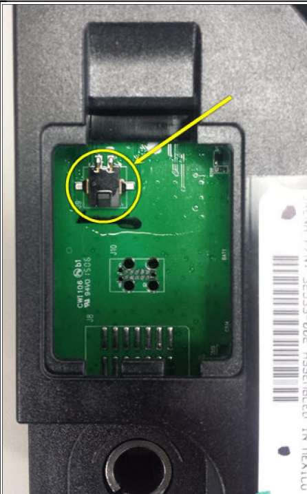
Figure 13 - Battery Cover Removed
