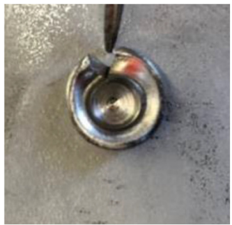
OK Rivet with 1 crack
