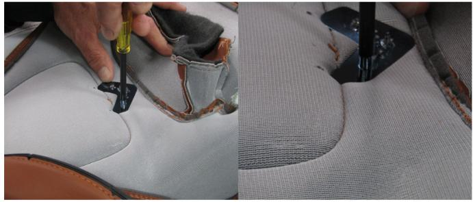
5. Using a 4 mm nut driver, slowly push down on the retainer plate until each pin on the emblem is fully seated in the retainer plate.
