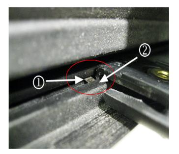
**Important:** Before attaching the front bar screws, inspect for proper installation of the sunshade within the track. When properly installed, the metal coil on the end of the sunshade (1) is BELOW the track (2). The graphic below shows an example of incorrect installation; with the metal coil (1) positioned ABOVE the track (2).
