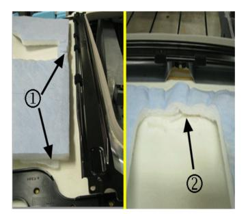
• Acoustic panels attached to the rear of the headliner may have partially detached (1) and/or bunched up (2) putting too much tension on the sunshade roller.
