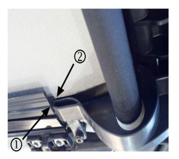
**Important:** As shown in the graphic above, ensure that the tab of each end cap is fully seated into the rail end (1), and that the sunshade material is properly positioned in the end cap and rail track (2).
