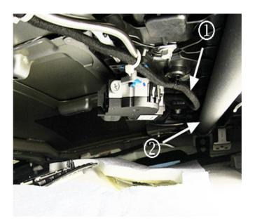
**Important:** While cycling the sunshade, closely inspect for possible contact/interference between the motor wiring harness (1) and the sunshade rollo fabric (2). It contact is evident, install an additional tie strap to hold the harness away from the shade.
