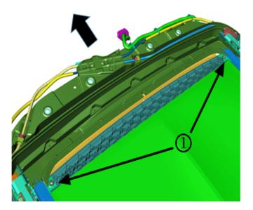
20. Install the screws (1) to the front bar of the sunshade and tighten to 2.5 N·m (22 lb in).
