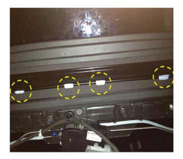
**Note:** The graphic above shows the current design crossmember, which has four hook and loop anti-rattle patches. The patches are shown blue in color on the above example to improve viewing. These patches will be black on the actual production crossmembers.
