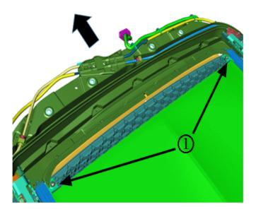
6. From the topside of the vehicle, remove the screw (1) from each end of the sunshade front bar that attaches the shade to the drive cables.
