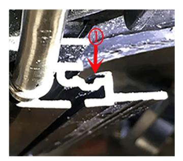
14. Locate the lower rail track (1) on one side of the sunroof housing.
