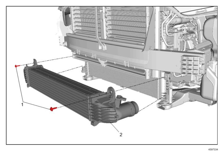
If you encounter a vehicle with the above concern, replace the charge air cooler. Refer to *Charge Air Cooler Replacement* in SI.
