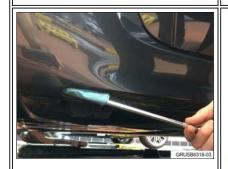
2. Attempt to clean the debris from the lens using a wet lint free cloth and low pressure water hose or spray bottle.
