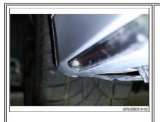
1. Using a flashlight, inspect the lens of the light carpet module from underneath the vehicle.
