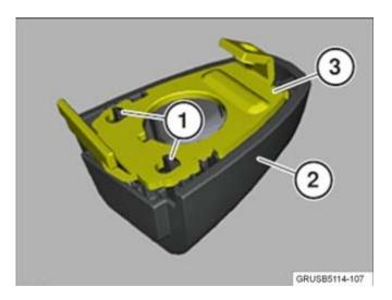
4. The latching mechanisms (1) of the cover (2) must not be damaged.
