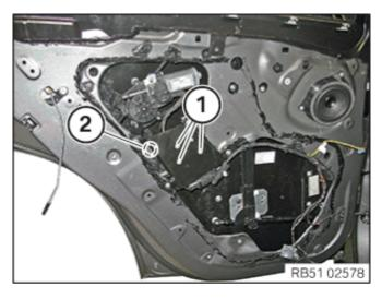
15. Remove the three screws (1). Unlock and disconnect the plug (2) on the drive unit, and carefully guide out the drive unit.
