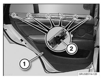
9. Carefully unclip the door trim panel (1) from the top retainers (2), and disconnect all plug connections.
