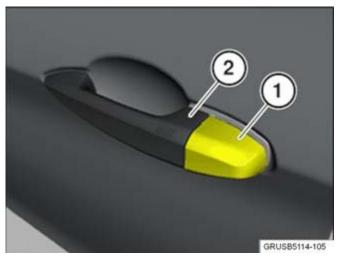
2. Pull the cover off (1) the door handle (2) by opening slightly.
