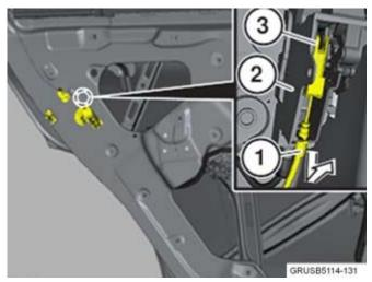
14. Disconnect the Bowden cable at the bottom (1) and top (3) from the door lock (2).
