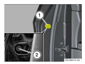
1. Pry out the trim cover (1) and remove the screw (2).
