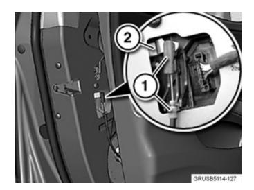
10. Unhook the Bowden cable (1) from the door lock (2).
