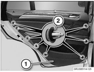
8. Unclip the door trim panel (1) from the clips (2) using special tool 00 9 325, starting from the B-pillar area.
