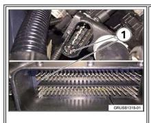
The fuel temperature/pressure sensor of the fuel supply line in the engine compartment is leaking at the connector
