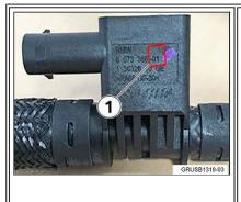
The improved fuel line can be determined by the change index (1) and part number located on the fuel temperature/pressure sensor of the fuel supply line.
