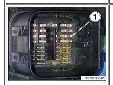
3. Check the DME and PDM connector sockets for coolant contamination (1).
