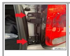
2. Visually inspect the mounting area of the tail light as shown to the left.
