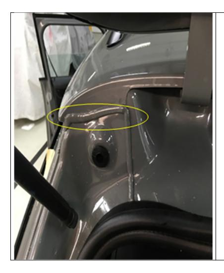
Visually inspect the body sealer at the top corners on both sides of the vehicle where the roof meets the D-Pillar in the area seen to the left.
