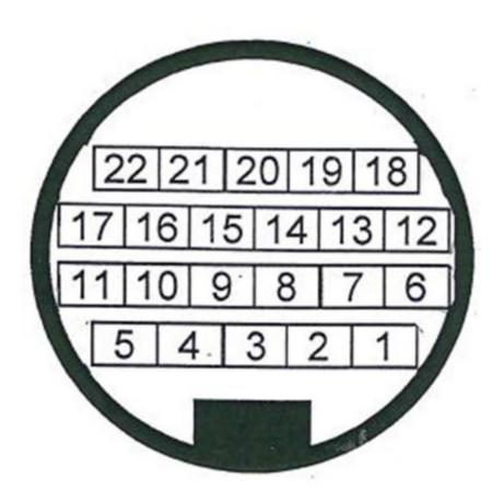
Note: When performing a pin drag test on the harness end of the transmission connector be sure t remove the TPA or you will get a false drag test as the TPA will also cause a drag on the diagnostic test probe.
