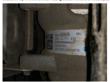
3. Torque Tube Casting Code
