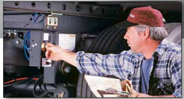
QUIK-DRAW allows drivers to disengage the slider's lock pins using only fingertip effort.
