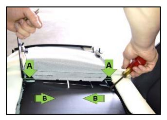
Fold the cover down and install the rear cover mount rod <arrow A> by using a pair of Pry Levers 80-200 (or equivalent) to gently compress the lumbar adjustment frame in the direction shown <arrow B>.
