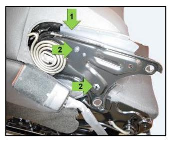
Reinstall the seatback trim plate <arrow 1> to both sides of the seat and ensure that the retainers <arrow 2> are seated properly.
