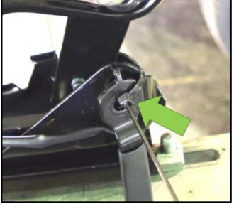
Secure the seat belt latch to the seat frame using a tie wrap or elastic cord as shown <arrow>.
