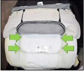
Fold the cover down and install the new upholstery clamps <arrows> using Upholstery Clip Pliers - VAG1634 (or equivalent).
