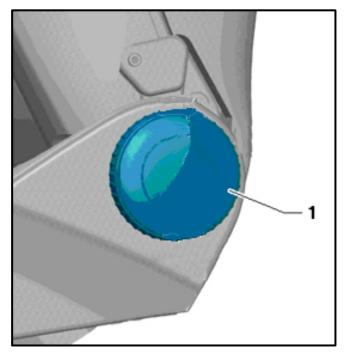
• If equipped, reinstall the backrest adjustment wheel <1> (replace the wheel if it is excessively loose after installation).
