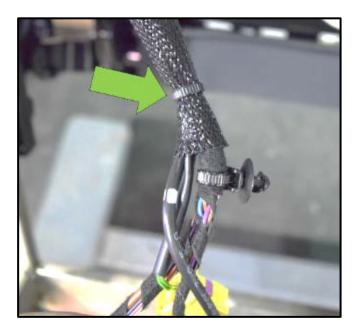
Secure the lower end of the wiring harness sheath at the location shown using a tie-wrap <arrow>.
