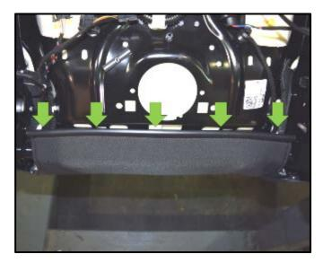
• Release the lower seat cover channel from the seat bottom pan <arrows>.
