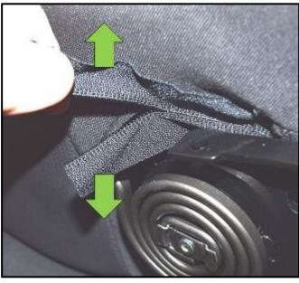
Once the ends of the seatback zipper have been extracted, carefully separate the zipper by pulling both halves in the directions shown <arrows>.
