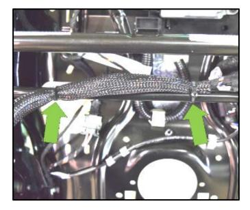
Secure the wiring harness sheath to the seat frame at the locations shown using two tiewraps <arrows>.
