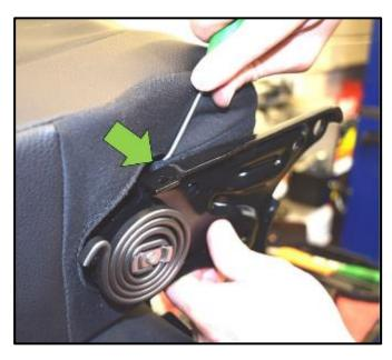
Using a small screwdriver (or equivalent) extract the end of the seatback zipper on both sides of the seat <arrow>.
