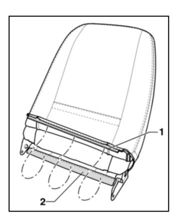
• Release the contact surface <1> from the mount <2> on the back side of the seatback.
