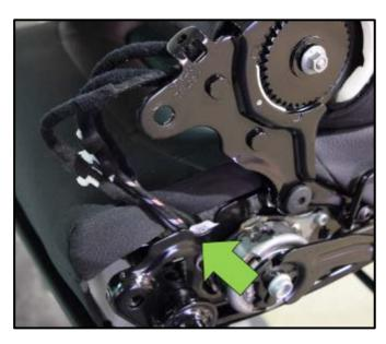
Properly route the seat and airbag wiring harnesses through the seat bottom <arrow>.
