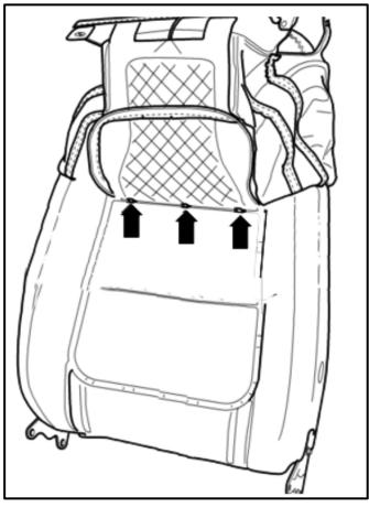
Fold the cover up and pry the cover profile out of the cushion mounts <arrows> using a small screwdriver (or equivalent).
