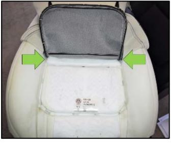
Fold the cover down and install the new upholstery clamps <arrows> using Upholstery Clip Pliers - VAG1634 (or equivalent).
