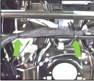
Carefully cut the two tie wraps from the seat frame and wiring harness sheath <arrows>.
