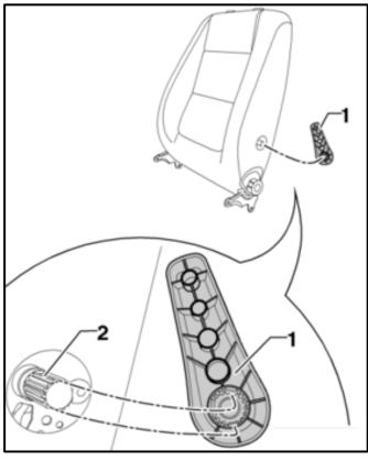
If equipped, pull outward on the lumbar adjustment lever <1> and remove it from the shaft <2>.
