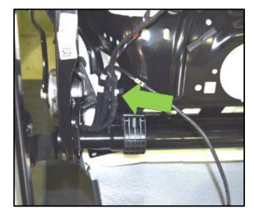
Reattach the wiring harness retainers located in the area near the seatback hinge <arrow>.
