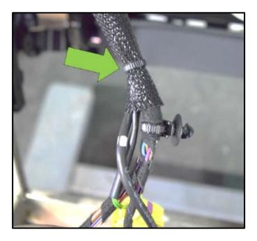
Secure the lower end of the wiring harness sheath at the location shown using a tie-wrap <arrow>.
