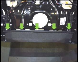
• Reattach the lower seat cover channel to the seat bottom pan <arrows>.
