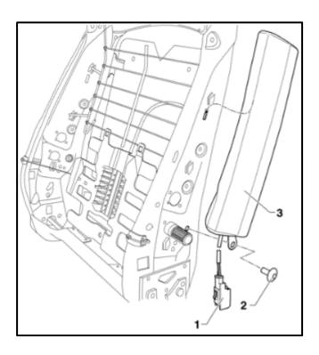
• Install the replacement side airbag <3> to the mount in the backrest frame.
