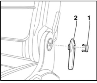
• If equipped, reinstall the release lever <2> and then the release lever cap <1>.
