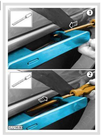
Use a suitable file to apply gentle upward force while sliding the file forward and then backward.
