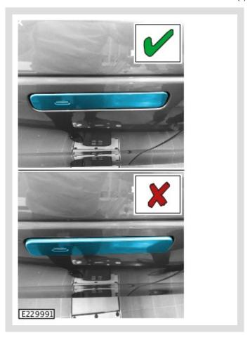
Lock the vehicle and inspect the position and operation of all exterior door handles.
