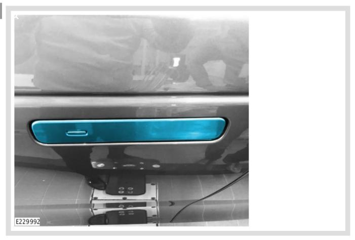
Lock the vehicle and inspect the position and operation of the reworked exterior door handles.
