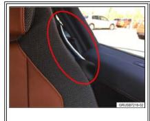
Friction between the contact points of the safety belt guide cover and the safety belt guide carrier plate which is attached to the backrest (general location is circled).
