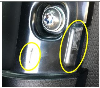
3. Apply film tape 83 19 9 407 798 to the carrier plate at the contact points (arrows/circled).
