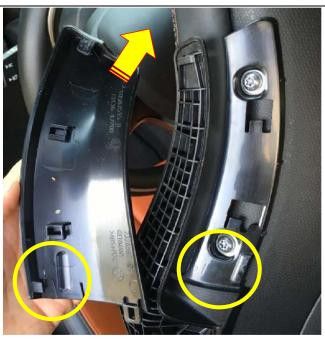
1. Remove the safety belt guide trim by carefully prying upward and outwards from the outer edge with a suitable trim removal tool.
