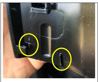
2. Look closely for material abrasion (circled) on the belt guide trim and on the carrier plate.
