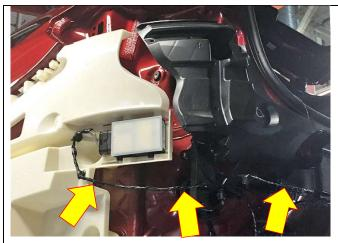
5. Check the routing of the harness for the rear side radar sensors.
