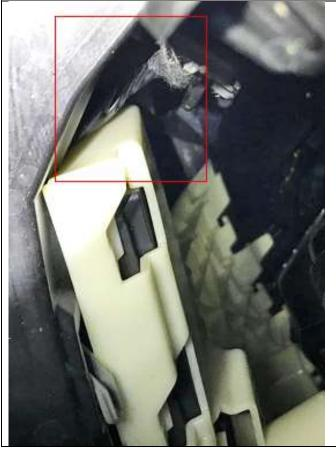
Harness can also run upwards and be pinched at the edge of the sensor mount (circled).
