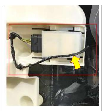
**Incorrect:** Harness runs upward from the sensor, partially blocking the signal area of the sensor.
