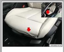
The upholstery of the sport seat adjustable thigh support may become exposed. The protrusions (general location indicated by arrow) can occur on either front corner of the seat thigh support.
