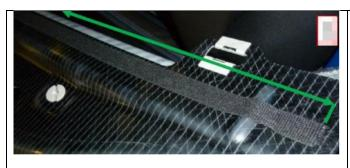
3. Close-up shows how the felt strip goes over the stiffening ribs.
