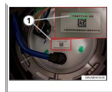
Check the part number of the fuel delivery unit (1). Compare the installed part number with the table below.
