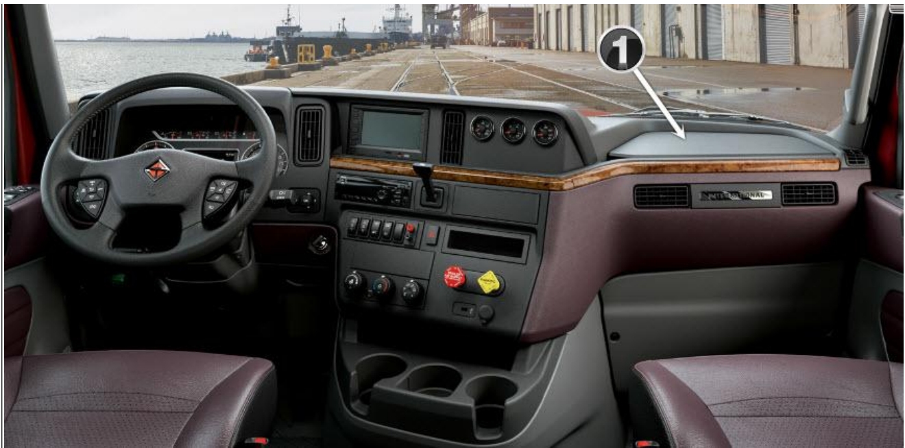
1. Fuse Panel Cover
