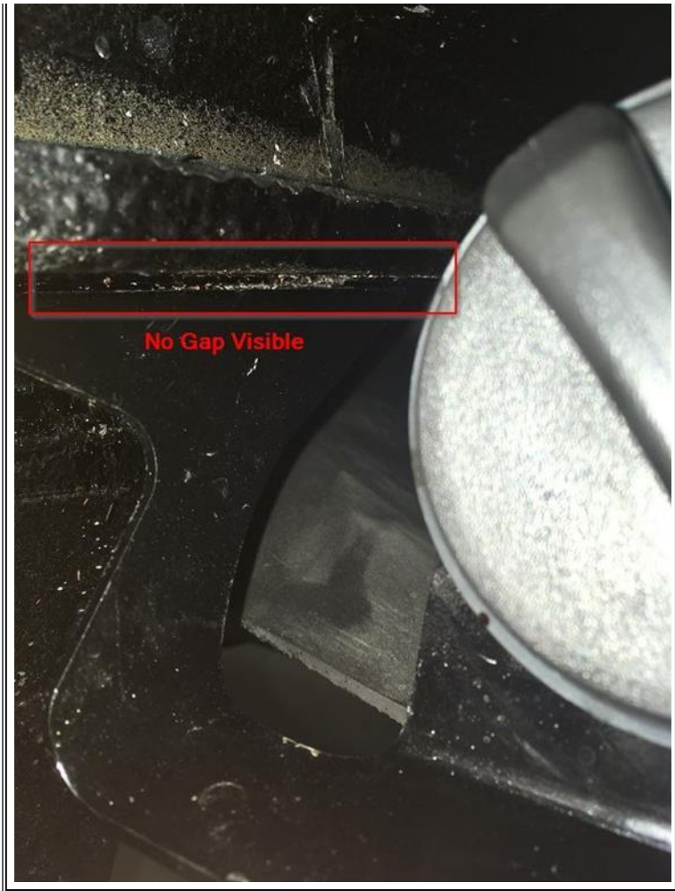
Figure 7 - Unacceptable Fill Receiver Bracket Gap
