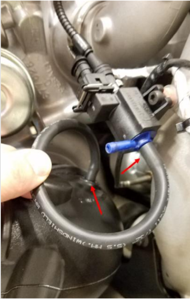
Figure #2: 12" Tubing Piece Connected
