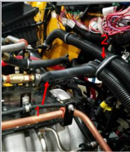
Figure # 1: Engine coolant supply hose
