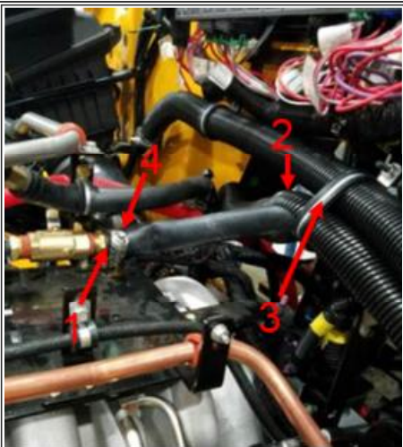
Figure # 2: Hose kink on supply line
