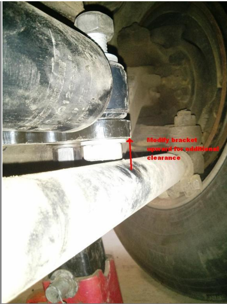
Figure 4: Tie rod tube to mount clearance
